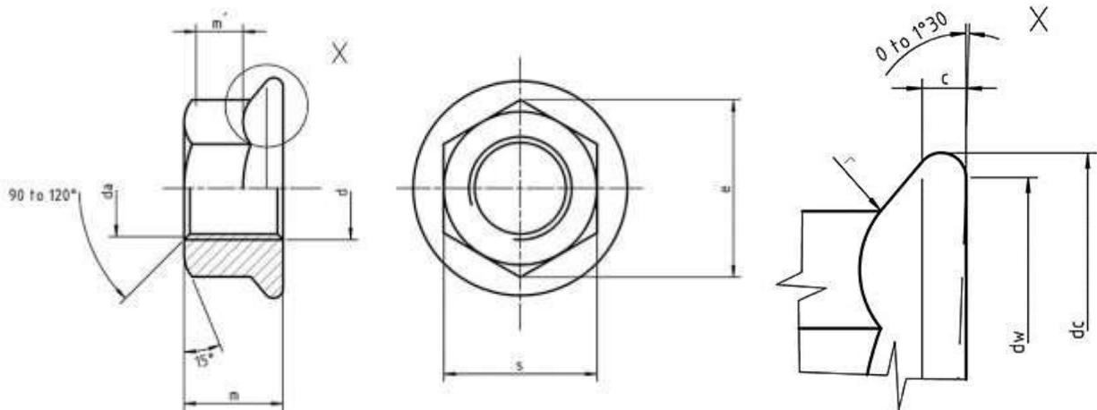
**Dimensions of Metric DIN 6923 Hexagon Flange Nuts**
